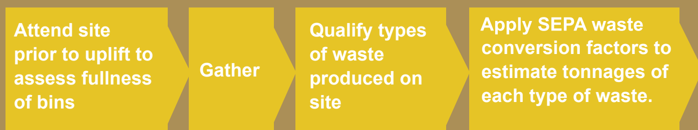
FIGURE. 11 PROCESS FOR ESTIMATING TONNAGE INFORMATION ON A SITE - BY SITE BASIS
