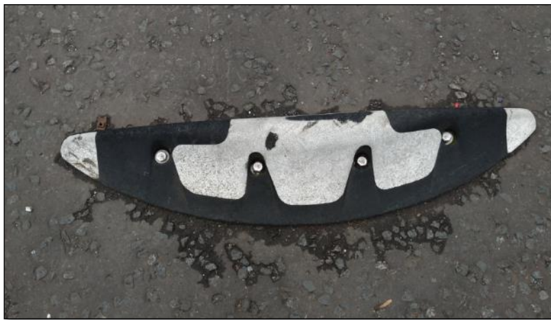
Figure 41: example of major damage to Orca on the River Clyde South Bank Route.
