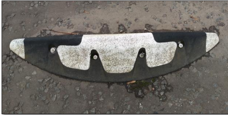
Figure 40: example of minor damage due to Orca on the River Clyde South Bank Route due to darkened surface.
