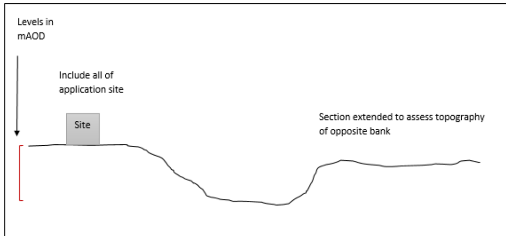
Figure 1. Example of appropriate site cross section.
