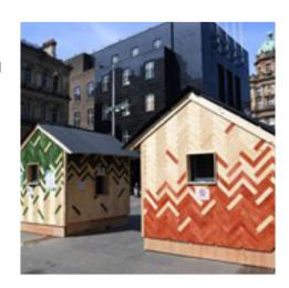
The results were staggering. All the ice had melted in the Scottish code box after just 11 days, while 121kg of ice remained in the Passive House box at the final weigh in on August 6.
