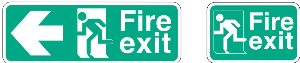
150 All fire safety signs, notices and graphic symbols should conform to the Health and Safety (Safety Signs and Signals) Regulations 1996. In addition to the fire safety signs specified in the Regulations, signs which conform to BS 5499-1:2001 will continue to satisfy the requirements of the Regulations.
