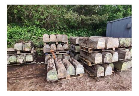
A recent example of this policy is the re-use of 90 metres of exquisite granite kerbing which once graced the western lawns of George Square. Many of the kerbs were two metres long and weighed 0.6 tonnes. This kerbing was saved during a redesign of the Square and stored in Victoria yard till a suitable project was identified, namely along the edge of the herbaceous border at Glasgow Botanic Gardens, directly opposite the Main Range of Glasshouses.
