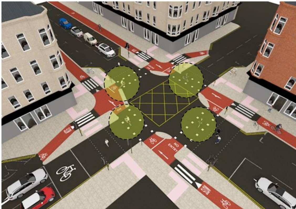
Figure 1: Cyclists using the protected cycleway to turn right at Allison Street junction
